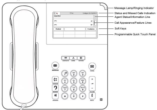
This phone supports 24 programmable call appearance/feature buttons. The labels for 6 of these buttons are visible on the main display and can be controlled by the adjacent buttons to the right. You can use the  $\triangle$  up and down  $\nabla$  arrow keys to scroll the display. You can also use the  $\triangleleft$  left and right  $\triangleright$  arrow keys to move through the button features in pages of 6.
